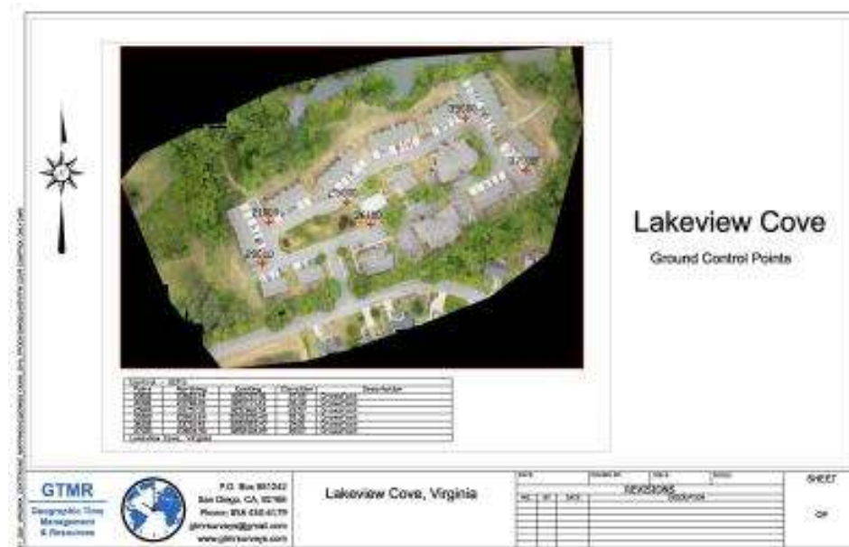
Ground Control Points (GCP's) for UAS / Imagery Operations
